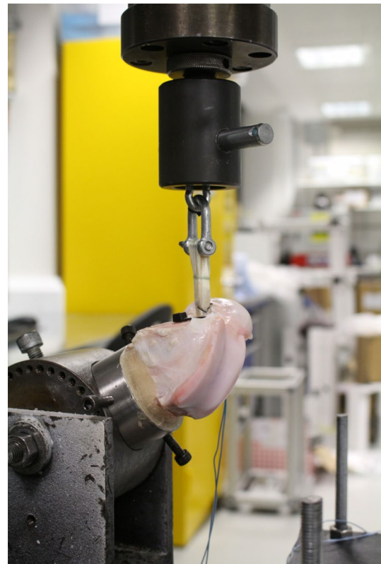
Fig. 4 In vitro ACL reconstruction simulation: a quadrupled peroneus longus allograft mounted within a porcine femur with the bone tunnel aligned to the loading axis of a servohydraulic Instron 8874 materials testing machine
